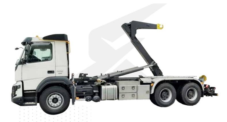
The **telescopic and articulated jib**, combined with the Marrel exclusive tilting frame, results in a reduced loading angle by up to 10° for maximum efficiency.
