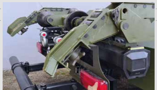
Patin de guidage stocké - twistlock arrière Rear roller support stored - Rear twistlock
